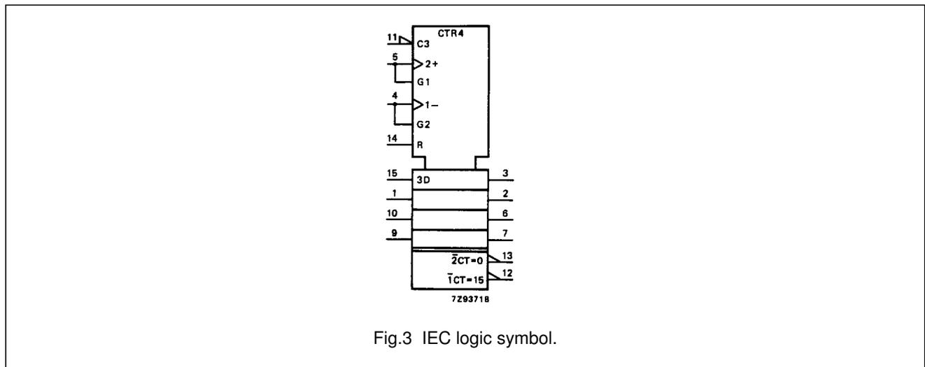
Pre-settable synchronous 4-bit binary
