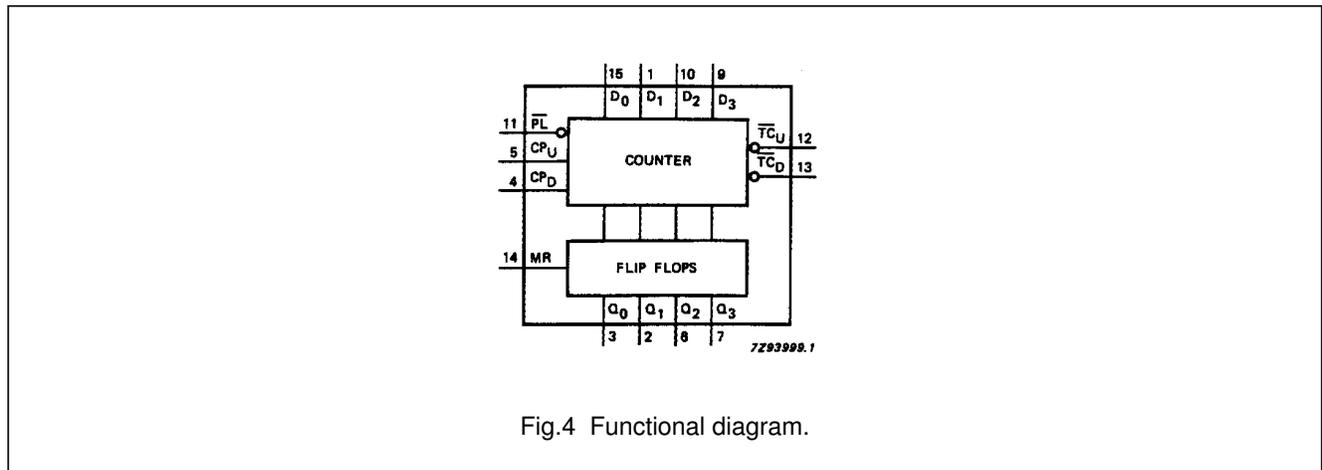
Fig.4 Functional diagram.
